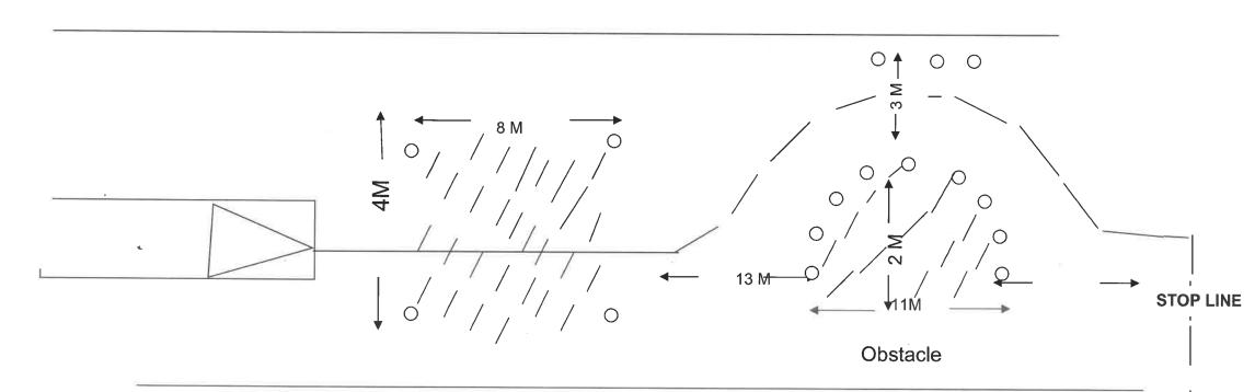
When passing between the first cones, the clutch pedal must be activated and Reducing of speed by the brake pedal and after passing the next cones the obstacle must be avoided by steering control. When passed the obstacle, the vehicle must be brought to a Full stop.
